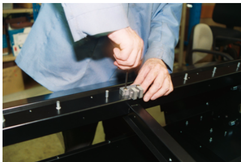
Figure 7: Loosening the Panel Hinges
